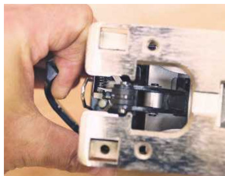
▲ The blade is secured into the shaft with a clamping action
